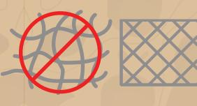
Tie wires should be used to prevent face bulging
