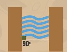
Internal baffles should be perpendicular to the slope and water flow
