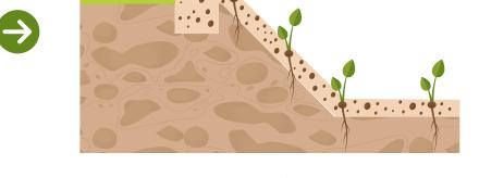
Made of photo/biodegradable materials, erosion control blankets eventually break down
